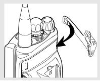
2 Snap the larger end of the adapter into place in the shroud indent, below the antenna port.
